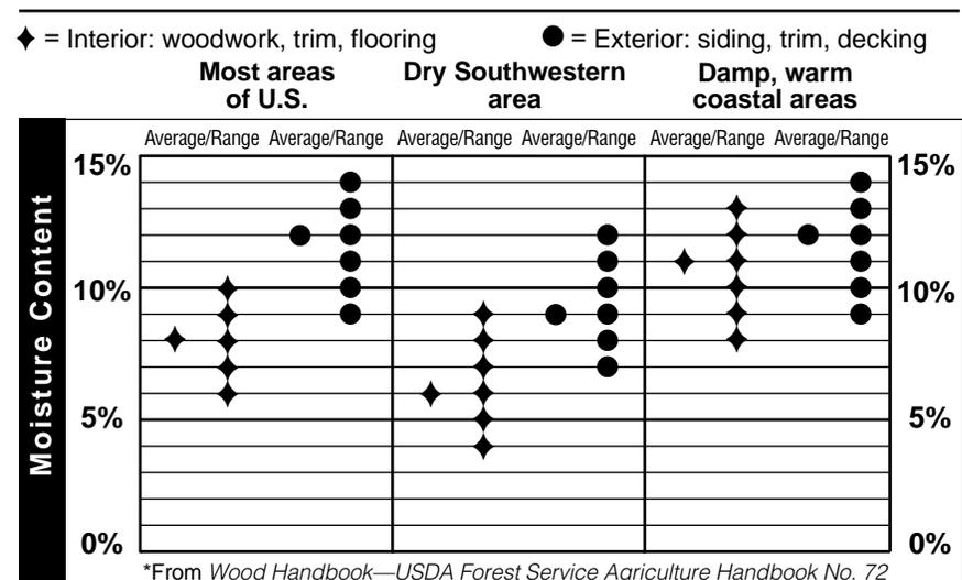
**Moisture content critical at time of manufacture and installation. . .**
