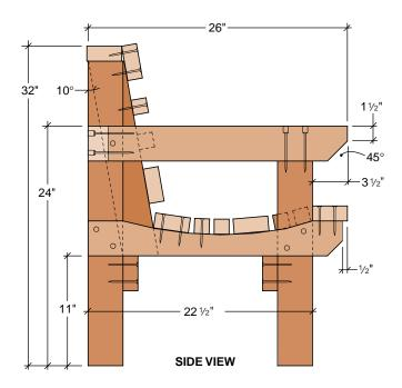
**4. Seat supports** The curved seat supports are made up of 2x4 lumber sandwiching either the 4x4 rear legs or the single 2x4 backrest support. To shape the curve, make a template for a 36-inch radius cut. Mark the cut to start 3 inches in from the front. Use a bandsaw to cut the radius to a depth of no more than 1½ inches. Finish the seat supports with a 45° bevel cut to match the armrests.
